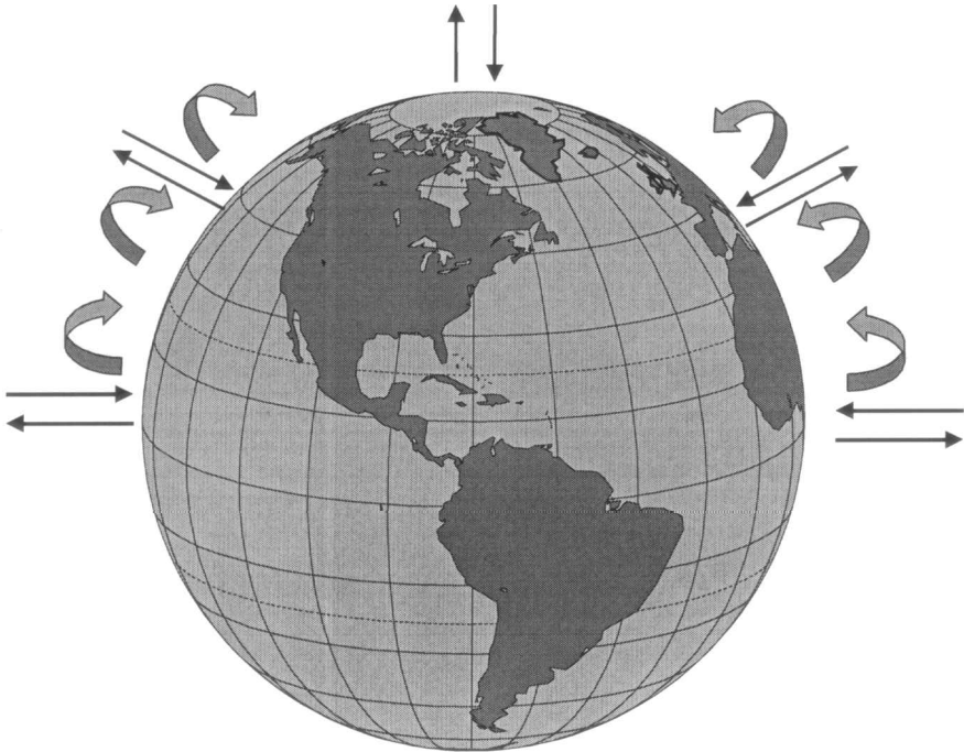
FIGURE 11. Illustration of the movement of persistent organic pollutants according to the global distillation hypothesis.
